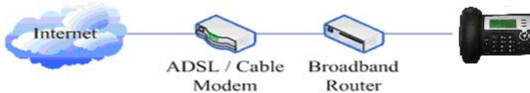
Shared network connection—Use this method if you have a single Ethernet port in your workspace with your desktop computer already connected to it. First, disconnect the Ethernet cable from the computer and attach it to the WAN port on the back of your phone. Next, use the Ethernet cable in the package to connect LAN port on the back of your phone to your desktop computer. Your IP Phone now shares a network connection with your computer. The following figure is for your reference.
